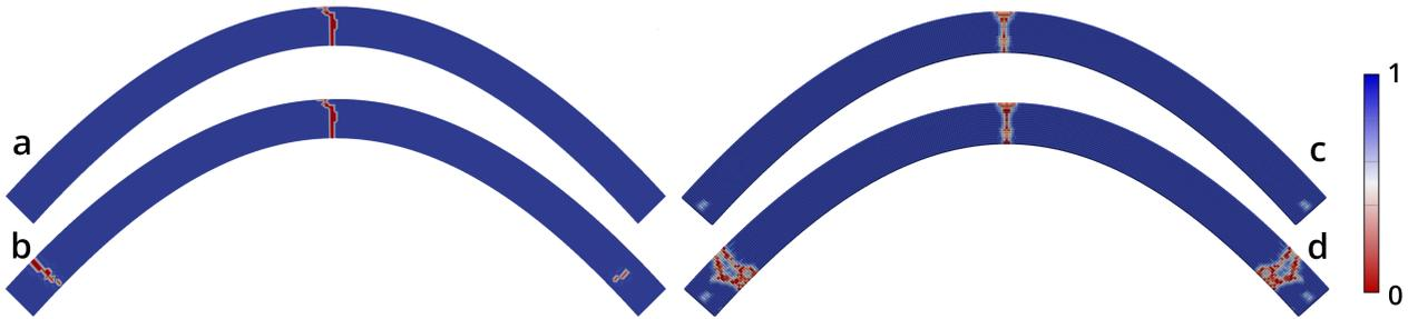
**Fig. 2:** Damage of a 2d curved bar; a, b: FE-approach; c, d: continuum-kinematics based peridynamics. The setup for the benchmark including loading conditions and material parameters is given in [9] for the FE-approach and in [11] for the continuum-kinematics based peridynamics approach.
