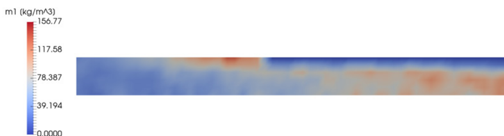
Fig. 1: Snapshot of the mass of crystalline aspirin in a flow tube crystallizer, due to attachment growth of dissolved aspirin from the surrounding fluid. The flow is from left to right, the upper boundary is a solid wall, and the lower boundary is the symmetry axis.
